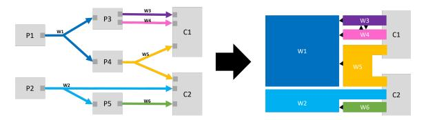
Table 5.36: A schematic illustration of the platform reduction process. The picture on the right features the original Platform instance with Producer instances P1 to P5, Consumer instances C1 and C2 and Connections W1 to W6. The corresponding Reduced platform instance is depicted on the right, with W1 to W6 now referring to Conductor and C1 and C2 to Reduced Consumer instances. The notation Wi  $\triangleleft$  Wj indicates that Wj may reference Wi.
