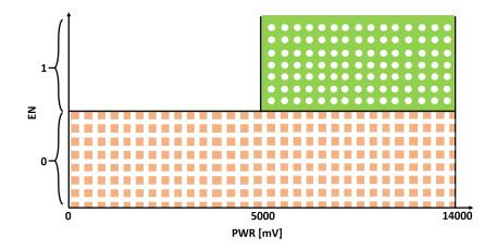
Figure 7.2: Simplification of the MAX15301's State Possibilities possible on the Enzian
