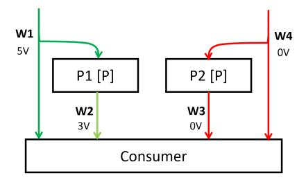
Figure 5.16: A Platform instance illustrating the issue of a transiently available bus
