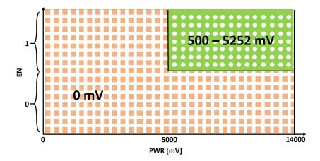
Figure 5.3: The relation between EN, PWR and OUT as a level plot
