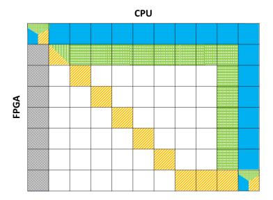
Figure 9.5: A visualisation of the different interleavings: With the interleaving our implementation normally prefers in orange (striped), said we encourage with our changes in blue and the one implemented in the existing management solution in green (dotted). Grey field with grid pattern mark impossible states.
