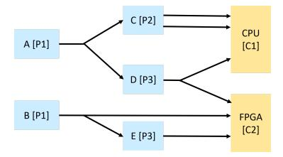
Figure 5.1: A schematic example of a platform instance, with producer and consumer instances drawn as boxes and the composition information abstracted as black arrows.
