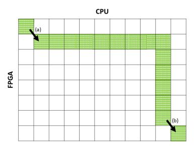
Figure 9.7: The manual boot sequence with the clock configuration step labelled with (a) and the phase-locking check step labelled with (b)
