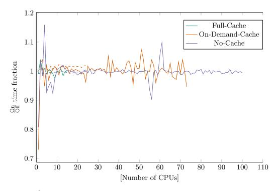
Figure 8.2:  $\frac{On}{Off}$  state generation time ratio. Dashed lines show data from Schibenstoll01, the undashed lines are from the Precision desktop dataset. We observe that there is almost no consistent difference between generating an "On" vs an "Off" state, barring values we can confidently consider noisy.
