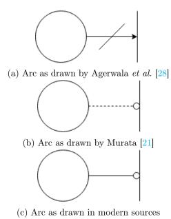
Figure 6.1: Inhibitor arcs in three styles
