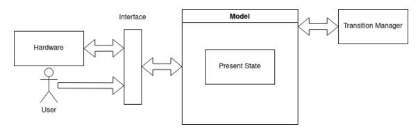
Figure 7.6: A Transition Manager is in charge of ensuring that the platform transitions from one state to another. It keeps track of the transition progress and future transition targets.
